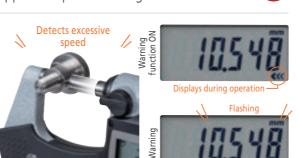
The approach speed warning function detects collisions with workpieces due to excessive speed. Even inexperienced workers can obtain stable and accurate measurement results.
