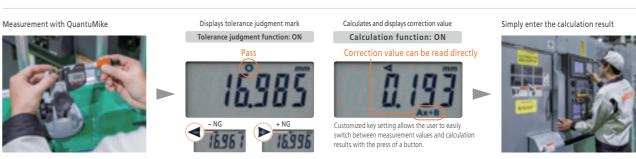
The micrometer determines whether the measurement value is within the upper and lower limits of tolerance and displays a tolerance judgment mark. The user can judge pass/failure at a glance.
